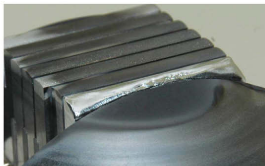
Fig. 4. Partially molten mini-prototype after exposure to a TEXTOR plasma ( E_{dep} > 130 \text{ MJ/m}^2 on front side).
